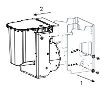
3. Using the installation template supplied (part no. 05-10-0011), drill 4 holes for M10 screws on the hull surface against which the fixed chassis is mounted. Screw in the fixed chassis in the order shown, using M10 screws. The recommended tightening torque is 33 N·m, to be adapted according to the hull type.
