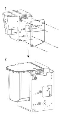
2. Remove the fixed chassis from the mobile chassis by unscrewing the parts shown in the diagram (4 M10 screws, 2 on each side). Keep screws and bolts aside.
