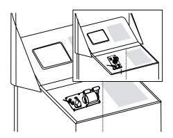
The Command Panel must be installed on the steering station, close to the multifunctional display, as shown.
