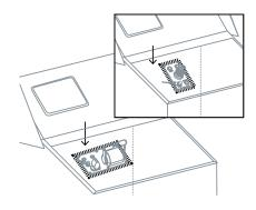
**5.** Screw the panel of the Command Panel. Use M5 screws adapted for the mounting surface. See p.5..
