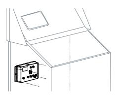
**2.** On the steering station, drill a suitable cable entry space for the wiring of the Command Panel.
