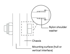
Galvanic corrosion is a common phenomenon in metallic structures that causes significant damage. This electrochemical reaction occurs when two dissimilar metals come into contact in a conductive environment such as a liquid, a soil or within atmospheric humidity.
