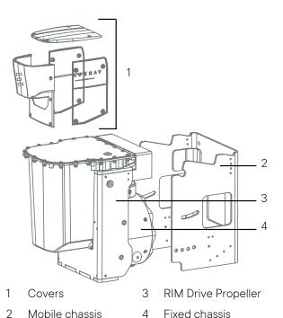
The Outboard Propulsion Unit of the BlueSpin system is designed for an outboard installation, against the hull.
