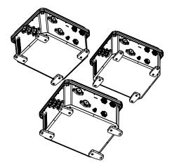
2. Screw the Power Unit into the chosen mounting surface. Use Ø<8mm diameter screws suitable for the mounting surface.
